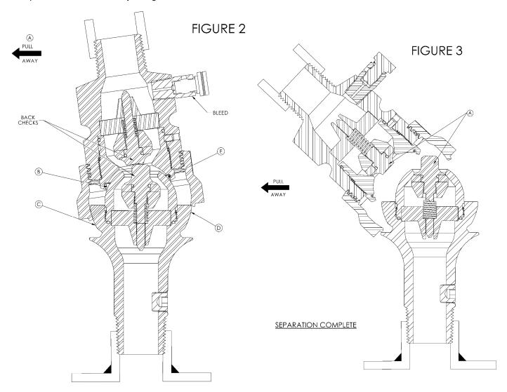
As the Tri Pod Upper Housing pivots, the catch nut will rotate out of contact with one or two of the three Tri Pod legs ①. While rotation is occurring the O-Ring ② on the Inner Ball Socket ③ maintains the product seal until release occurs. After a maximum rotation of 25 degrees, the Tri Pod Upper Housing ① and Catch Nut Assembly ⑤ will separate from the Lower Housing Assembly ⑥.
